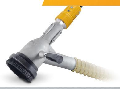
A dust-free abrasive blast system includes a combined blast and vacuum head BSH, fitted with a nylon-bristle brush that presses against the blast surface. The BSH blast and vacuum head assembly comprises a blast nozzle and a vacuum hose, which evacuates dust and the rebounding abrasive following its contact with the blast surface. This BSH blast and vacuum head contains the abrasive and keeps the surrounding area clean.
