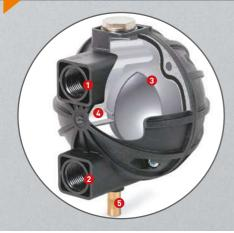
Drain is installed bellow pressure vessel, filter element, dryer, cyclone separator or similar pressure system element. Through G  $\frac{1}{2}$ " upper inlet port (1) on the top condensate accumulates in the drain reservoir (4).
