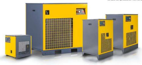
RDX-series refrigerated dryers with a capacity of 0.4–36.0 m3/min are equipped with an efficient cast-aluminium heat exchanger and an inbuilt coalescence separator. The low degree of pressure loss due to the inbuilt separator and the reliable outer insulation of the heat exchanger facilitate a high level of energy efficiency for the system. The coalescence separator is insensitive to pressure fluctuations in the case of varying load and reliably removes up to 98% of condensed moisture.
