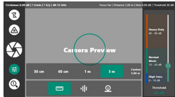
Figure 14: Adjusting the focus manually (example)
