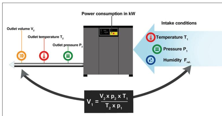
The delivery rate of compressors depends on the intake air.
